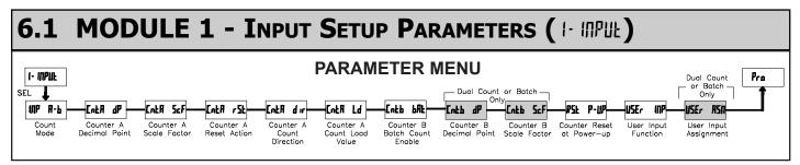
Shaded area selections only apply when Counter B is enabled (Dual Counter mode or batch counter).
