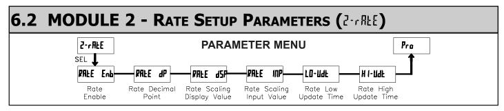
Module 2 is the programming for the rate parameters. For maximum input frequency, Rate Enable should be set to ND when not in use. When set to ND, the remaining rate parameters are not accessible. The rate value is shown with an annunciator of "P" in the Display Mode.
